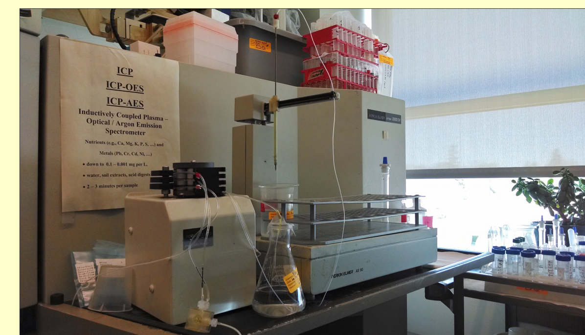
Figure 2. ICP/AES used for Mg and Ca analysis
