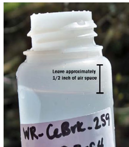
Figure 7: Leave 1/2 inch of air space
