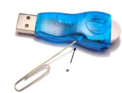
To eject iButton from USB adapter
