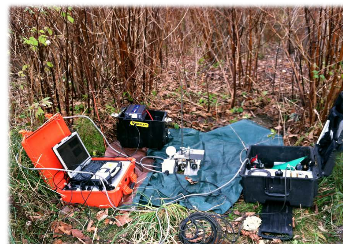
(Above) Pictured is the automated in situ BST machine mid test. The whole system includes the electronics case (orange), a portable battery, the BST machine (center), and the mechanics case (right). In the background you can see a dying grove of Japanese knotweed.
