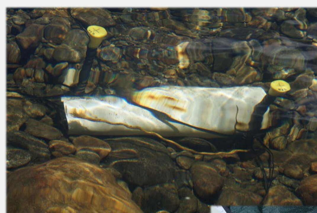
(Left) A pressure transducer is secured to the stream bed in a section of PVC pipe to safely monitor the stream height.
