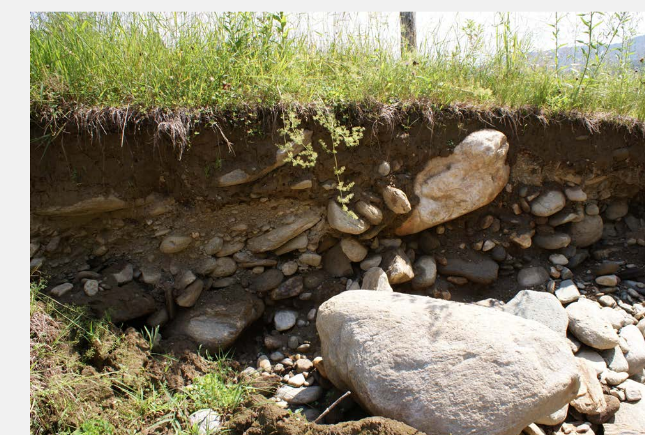
(Left) High levels of rock and gravel consistently prevented accurate strength tests to be conducted in areas of interest.
