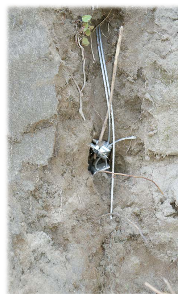
(Left) Here I am installing accelerometers on a stream bank that was displaying weakening conditions.
