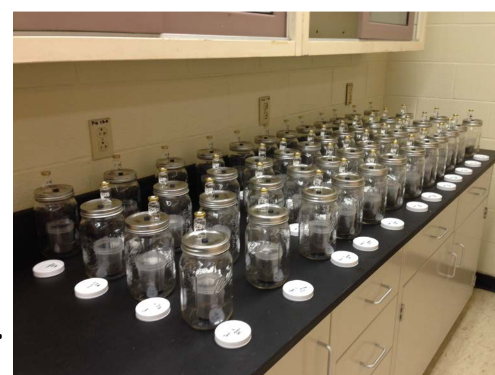
Figure 2. Incubation jar set-up
