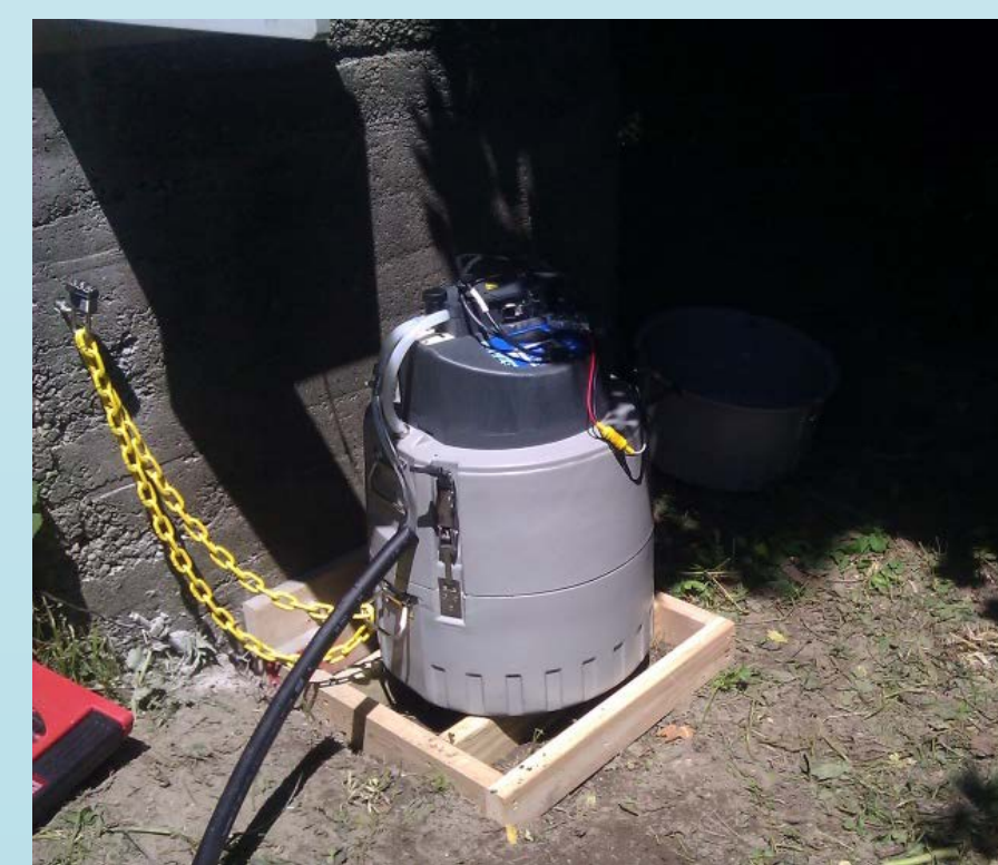
Figure 2: ISCO Automatic Sampler installed in Missisquoi
