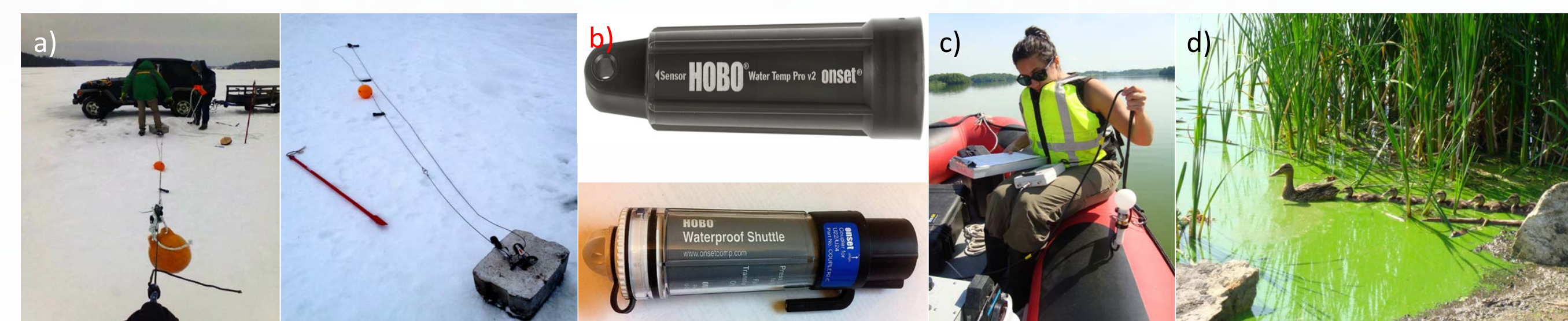
Figure 4. a) The thermistor chain comprises five temperature HOBOTemp Pro v2 u22-001 loggers and was installed when the pond was still frozen. b) Temperature HOBOTemp Pro v2 u22-001 loggers (top), and HOBOTemp Waterproof Shuttle data downloader (bottom). c) Collecting Photosynthetically Active Radiation during weekly sampling. d) Documented cyanobacteria bloom on June 17, 2014.
