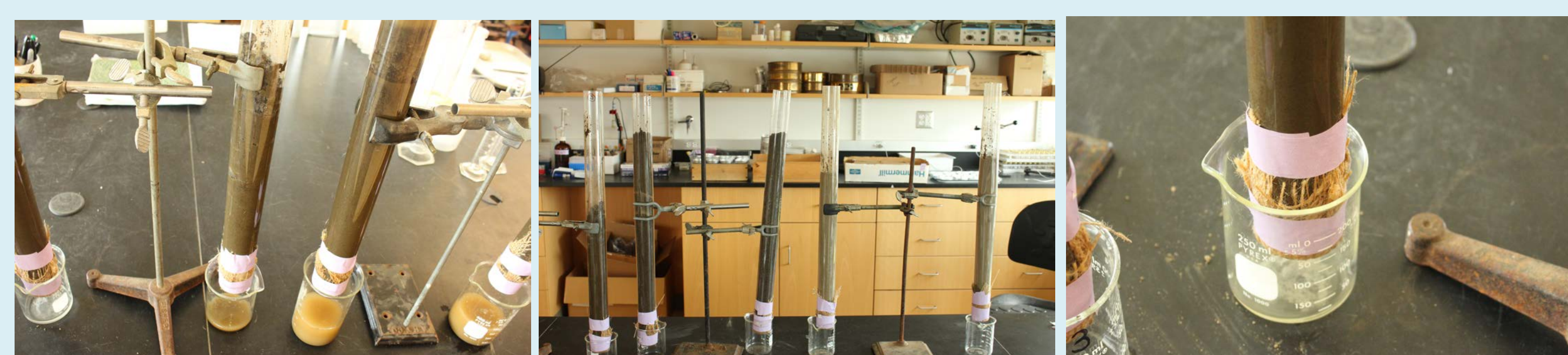
Figure 5: Experimental set up of soil column study
