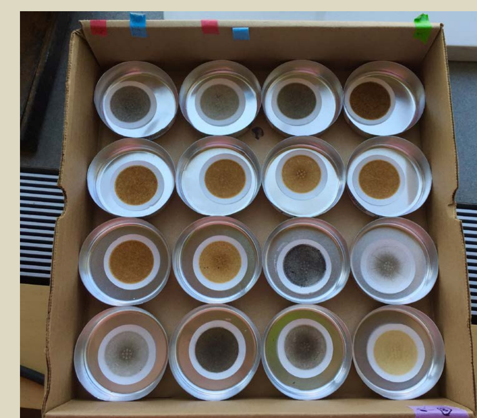
Figure 5. These TSS filters show solids after filtering water samples. Filters were dried and weighed to determine the concentration of TSS in the effluent.
