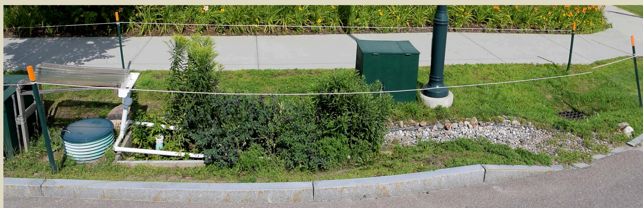
Figure 1. UVM Bioretention Cell 1 Stormwater runoff from the street enters the cell through the curb cut, then flows over the gravel pathway into the weir box where inflow samples are taken (shown on right side of photo). Runoff spills over a 90° V-notch weir to measure volume, and permeates through the cell. This cell is fitted with a rain pan, which mimics passive addition of rain and adds additional precipitation directly to the cell via the white pipes. Each cell is lined, directing all effluent to drain into an underground pipe where outflow samples are collected and volume is measured before it is released into the storm sewer. Control cells do not have a rain pan.
