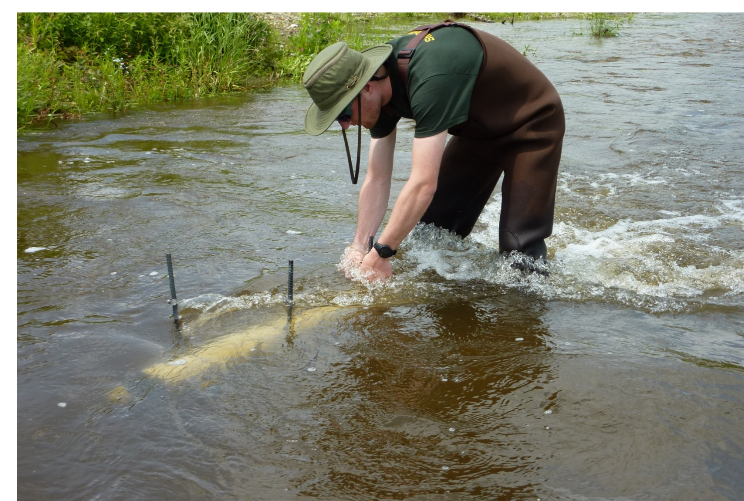
Figure (Left): Installation of Phillips Sampler at The Branch.
