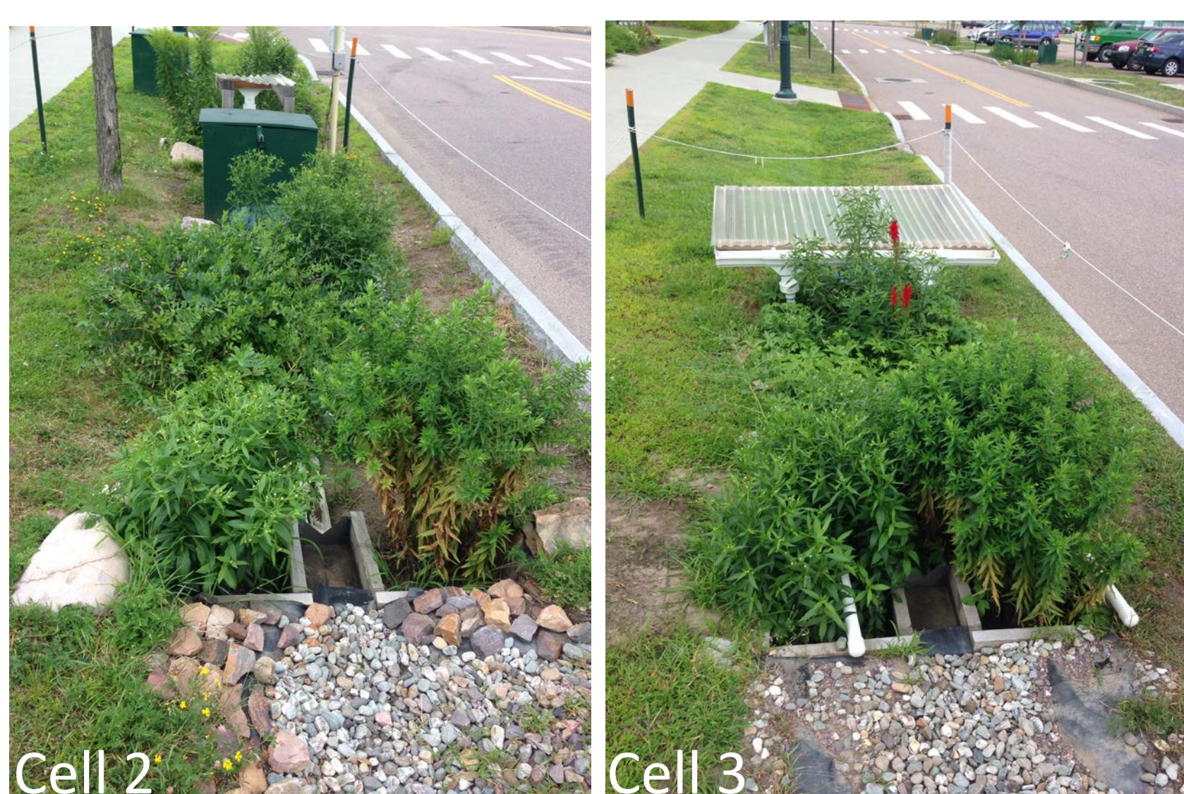
Figure 1. Cell 2 has typical bioretention soil and vegetative treatment. Cells 3 and 4, both containing Sorbtive Media Treatment, were different in that cell 3 has an additional rain pan.
