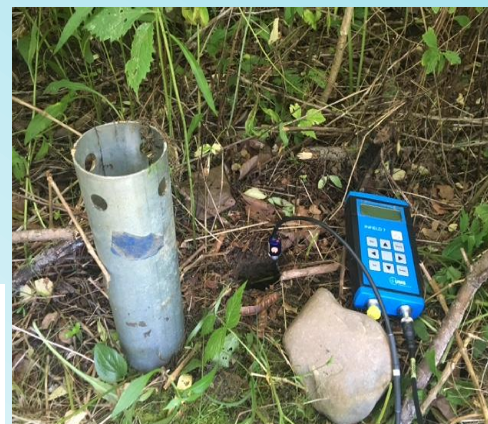
Figure 3. Recording matric suction readings from a "hole" sample at Lareau Farm, July 2016.
