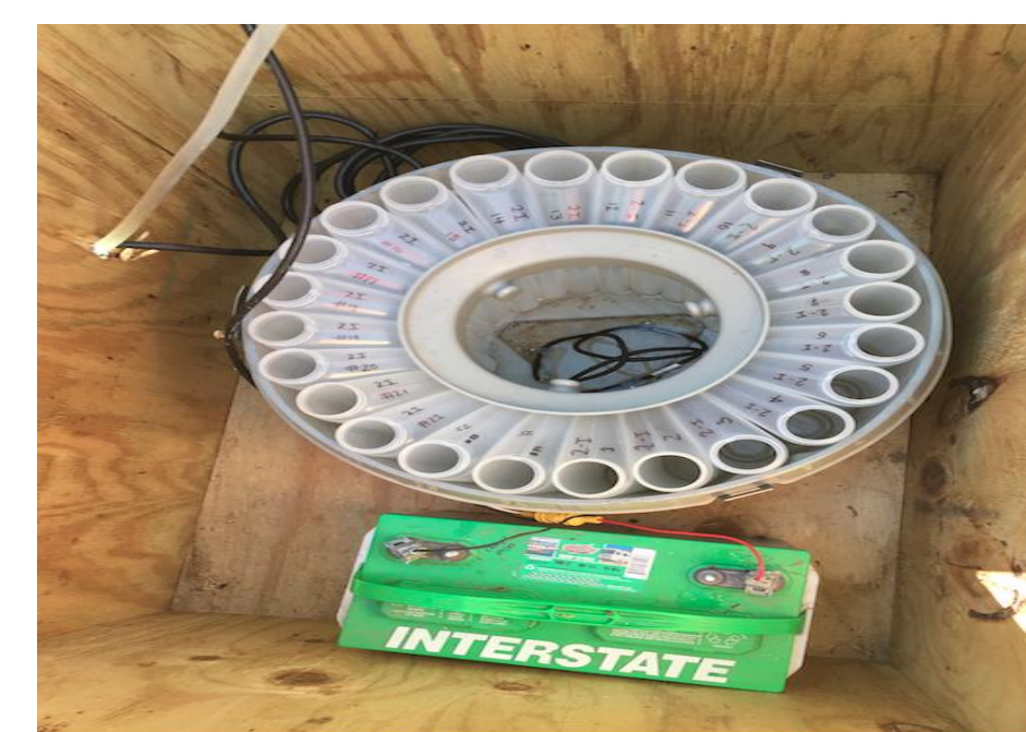
Fig. 3 ISCO auto-sampler used to collect effluent that has passed through the bioretention cell.
