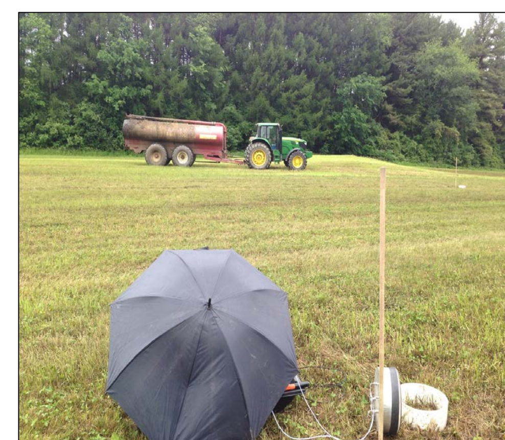
Fig. 1. Example of greenhouse gas sampling setup in Field 1 (BMP).
