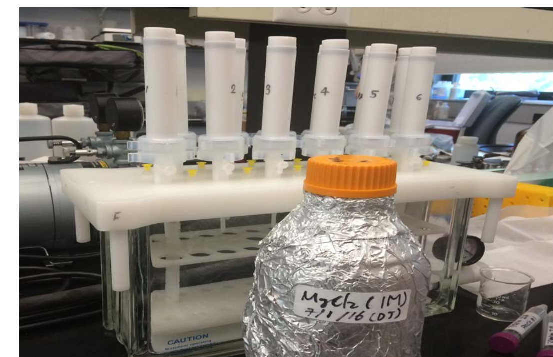
Fig 3. SEDEX extraction apparatus setup
