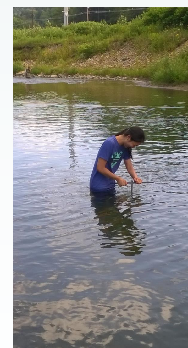
Figure 3: Auguring Sedimeter into the Mad River Bed
