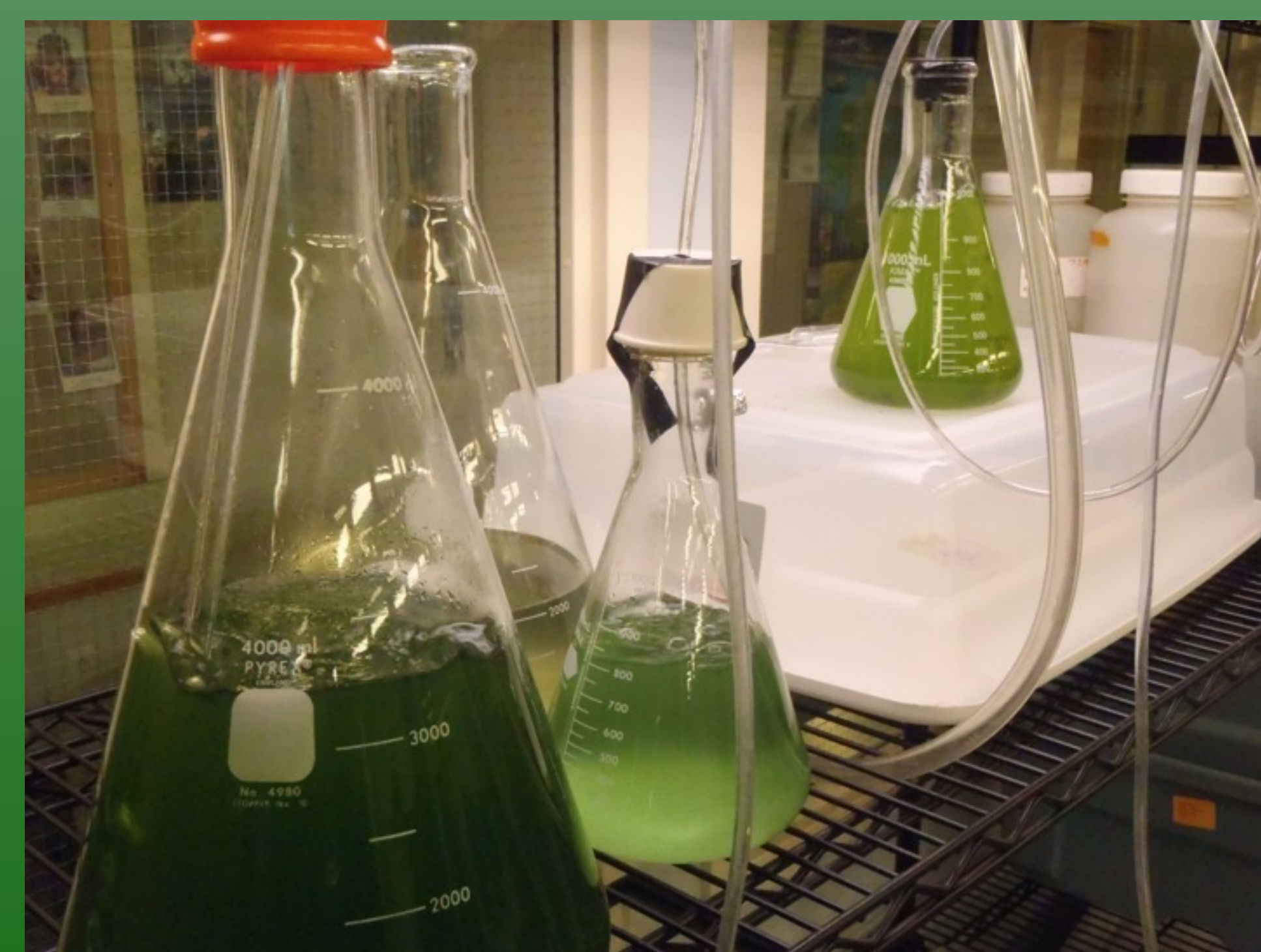
Figure 2. Beginnings of the Selenastrum culturing system.
