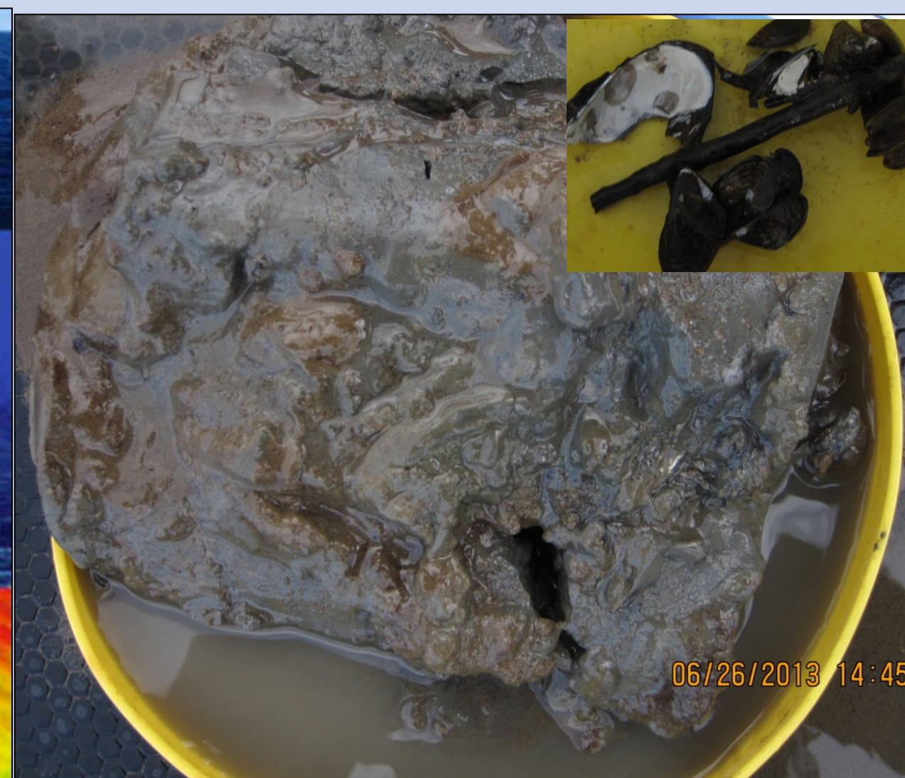
Figure 2: Shelburne Bay sediment grab sample with burrows, detrital matter, mussels, snails, a thin biological surface layer and a organic-rich bottom layer.
