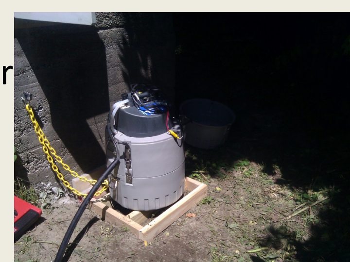
Figure 2- ISCO Automatic Sampler being installed in Missisquoi
