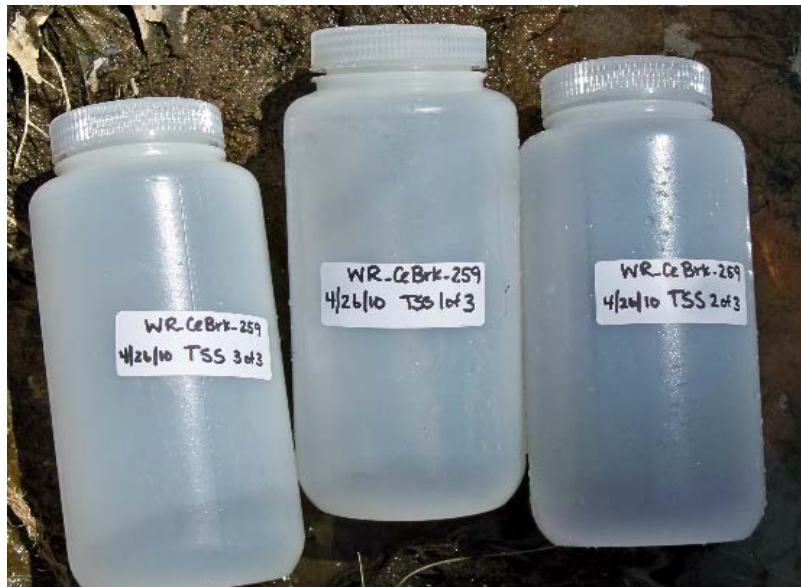
Figure 5: 3 Total Suspended Solids bottles (1L)
