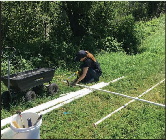
Undergraduate intern Sara Mecca saws a PVC pipe for the sensor installation. Sensors go in the pipes.
