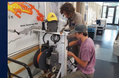
Undergraduate interns Bridger and Toby help hook-up the internal electronics for the water quality monitoring platform.
