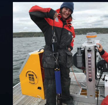
PhD student Wilton Burns hooks up the EXO sonde to the water quality monitoring platform. The sensors are attached via an orange cable and operated by a winch to make vertical profiles of the water column every hour.
